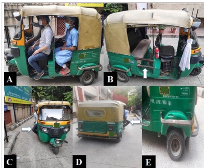
Figure 2: (A). An Indian tricycle (autorickshaw) with no doors/bars on the left side. The tricycle is overloaded with two extra passengers in the driver's (front) seat. (B). On the right side, the backseat is protected by bars (arrow) but the driver's (front seat) is open. (C, D). Right leg of the extra passenger sitting in the front seat protrudes out predisposing it to a sideswipe injury (arrows). (E). Iron angle over the rear wheel can dangerously hit the leg during a sideswipe.
